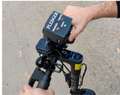
Figure 1: Alert notification gadget for UC2 mounted on an electric scooter. The green LED indicates readiness of the application and on-street radio connectivity.
