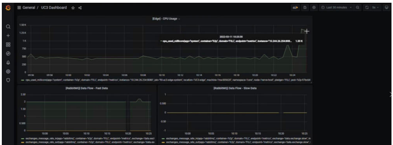
Figure 34: Grafana dashboard of UC3 for monitoring the infrastructure and performance of the service
